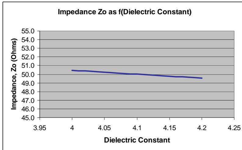
variation in dielectric constant and impedance for as typical polyimide product with nominal Dk of 4.1 and thickness of 0.010”) These relationships will always be similar when considering the sources of impedance variation within a given system, regardless of the absolute values of the variables.
