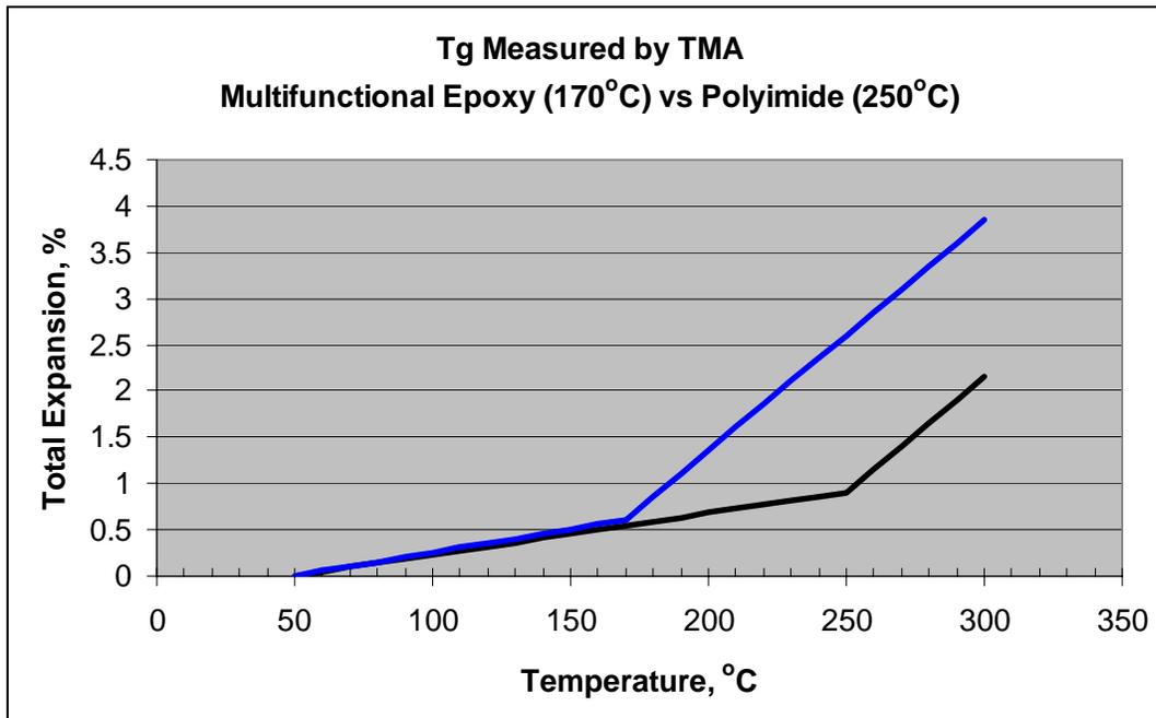
One of the most common results of the softening of the resin at its Tg is that it becomes easily smeared during drilling. With conventional FR4 the heat generated at the cutting surfaces of the drill is usually sufficient to cause smearing. In addition, when resin is heated above its Tg, either in use or during processing, it will cause substantial reduction in bond between the resin of the laminate and its copper foil cladding, resulting in pad lifting and other problems with surface features.
