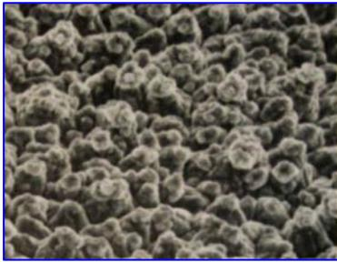
The "standard" copper treatment consists of microscopic copper nodules deposited over the copper "teeth" on the bath-side of the foil (see photomicrograph below). To reduce oxidation and make a more thermally stable treatment, brass, zinc or sometimes nickel is plated lightly over the deposited copper nodules. A further treatment in the form of a very light zinc chromate or other antioxidation treatment may be used to prevent oxidation of the drum or smooth side of the foil.
